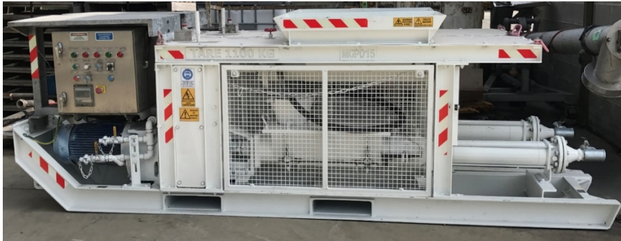
Figure 9: 1000 volt electric placer pump side view
