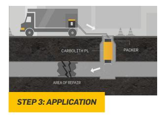
This packer is transported to the area of treatment and positioned in place using slide rods, pneumatic rods or a winch. Inflation of the packer presses the saturated fibreglass mat onto the pipe or sewer wall. The resin bonds the laminated fibreglass mat to almost all commercial pipe materials and thus permanently seals and repairs cracks, fissures, and otherwise damaged areas.
