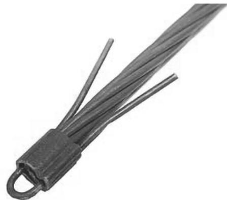
*Minova fishhook style cable system is swaged on with steel tubing and bent hooks can accommodate any size borehole, firmly holding the cable in place during the post-grouting process.*
