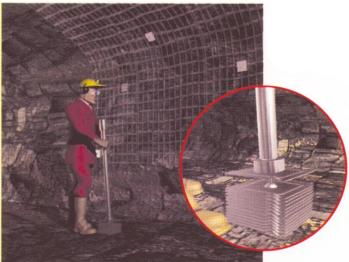
Miner picks up plate from carrying holder with magnetic end of installation tool.
