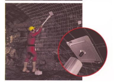
Installation tool is reversed, allowing miner To hammer plate tight with driving head.
